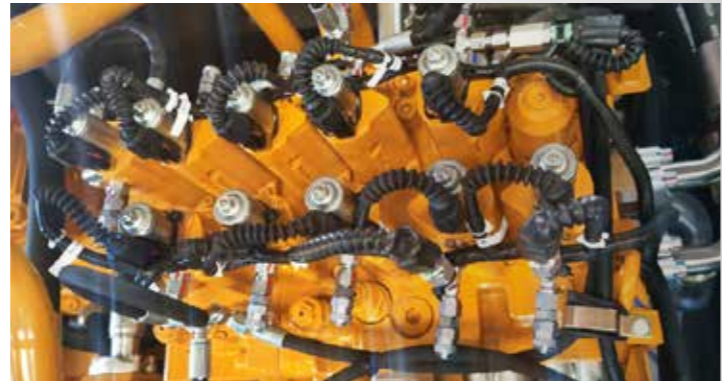
Kawasaki KMX36NAE electronic control main valve is a leader in the industry. Its flow capacity is 25% higher than that of 32NA main valve, which is more energy-saving. After one year, SANY and Japanese experts carefully carried out commissioning to make the coordination performance more excellent.
