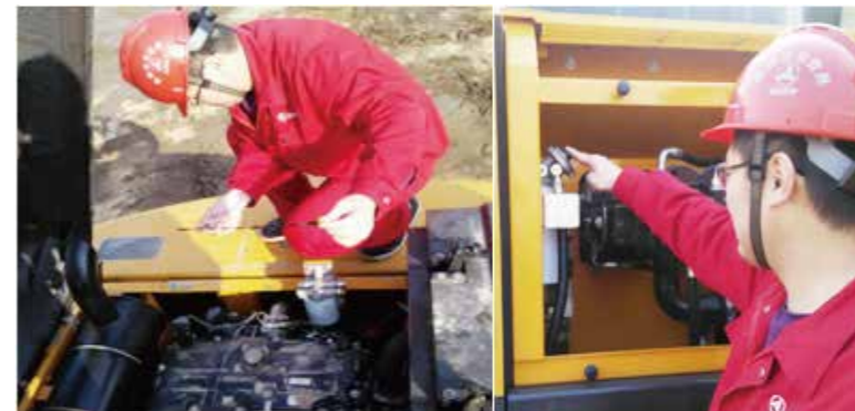
Inspect the situation of engine oil
